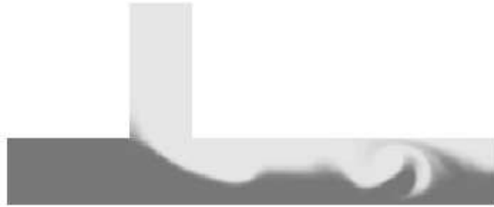
FIG. 4.3 – Instantaneous temperature fields in a 2D unsteady Tee junction at t = 12.2s (8 recirculation times) - non-physical temperature regions ( ie out of limits) are denoted by dark contours.
